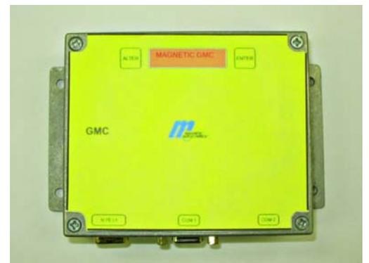
The Magnetic Gate Master Controller comprises a number of sub-modules when interconnected via an internal bus are able to control the operation of the gate via commands received from an external serial port or as a stand alone unit with a dedicated I/O module.
